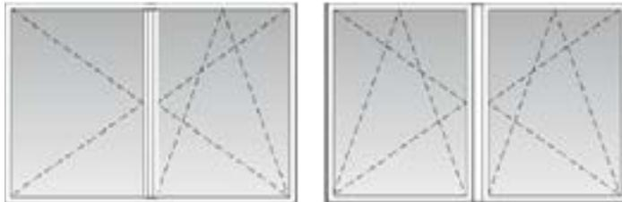
double frame window: side hung+side hung, tilt and turn + side hung, tilt and turn + tilt and turn
