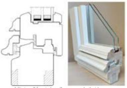
possibility to mill for window sills on one or both sides
