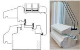
possibility to mill for window sills on one or both sides
