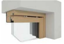
FLUSH TOP GUIDE BAR no protruding elements of fittings in the window lintel.
